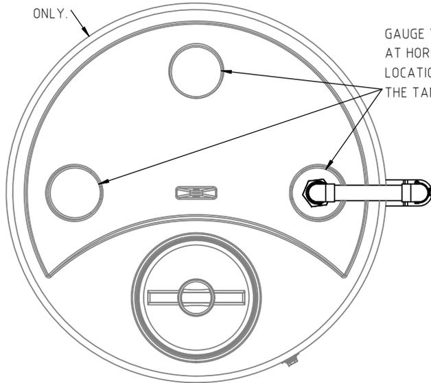
GAUGE TO BE INSTALLED AT HORIZONTAL FLAT LOCATIONS ON THE TOP OF THE TANK.
